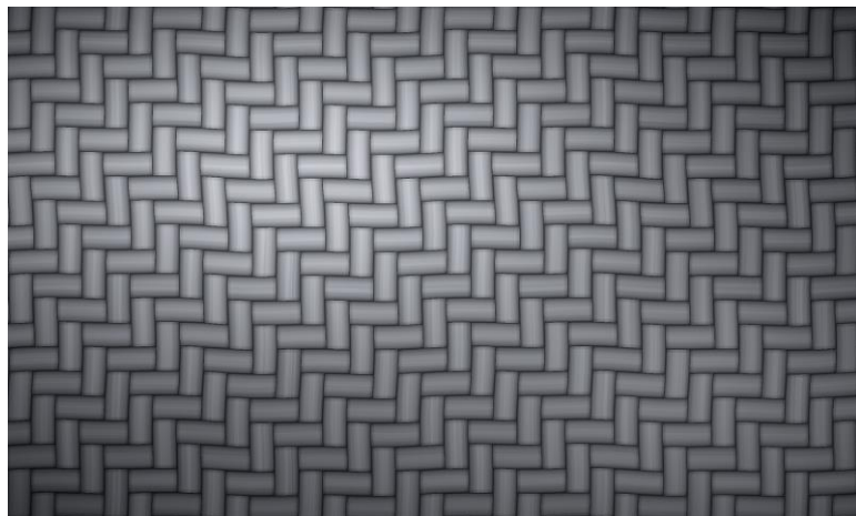
Figure 1. Close-up of a 2/2 twill carbon-fiber reinforcement of the type used in aerostructure skins and secondary structure. The architecture that gives the laminate its specific stiffness and strength is also what makes an irreversibly cross-linked matrix so difficult to separate from the fiber at end of life.
