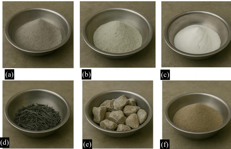
Figure 1. Composite material constituents used in the study: (a) Fly ash (FA), (b) Ground granulated blast furnace slag (GGBS), (c) Nano-silica (NS), (d) Basalt fibers (BF), (e) Recycled coarse aggregate (RCA), (f) Manufactured sand (M-sand).
