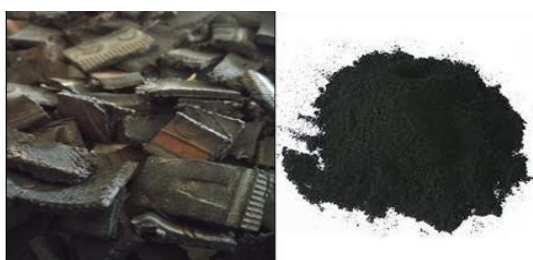
Figure 1. Rubber tyre chips (RTC) & Rubber tyre Powder (RTP)
