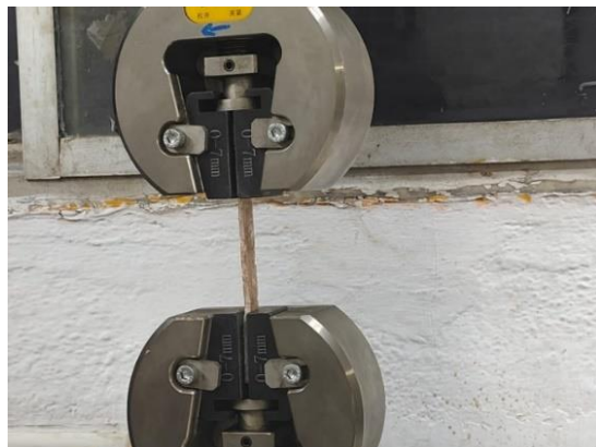
Figure 3. Photographic view of tensile test performed on specimen
