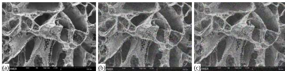
Figure 1. (a)–(c) Original polymer microstructure image (Leica Microsystems, cryo-BIB-SEM) and its Gaussian-noisy counterpart used for model evaluation. (a) Original polymer image; (b) Gaussian noise; (c) Salt and pepper noise.
