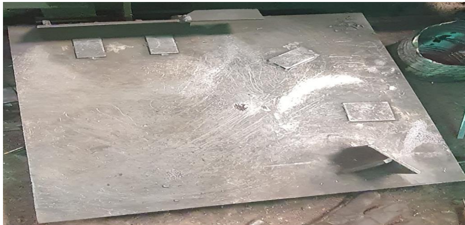
Figure 9: Support plates have been added to prevent workpiece misalignment and distortion.
