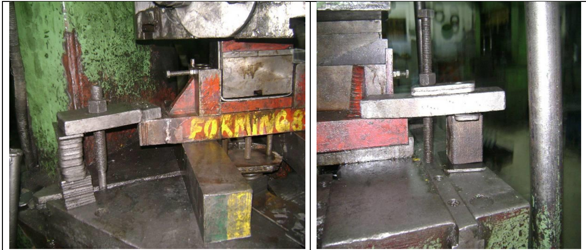
Figure 4: The introduction of clamping blocks instead of packing plates was implemented through the KAIZEN method.
