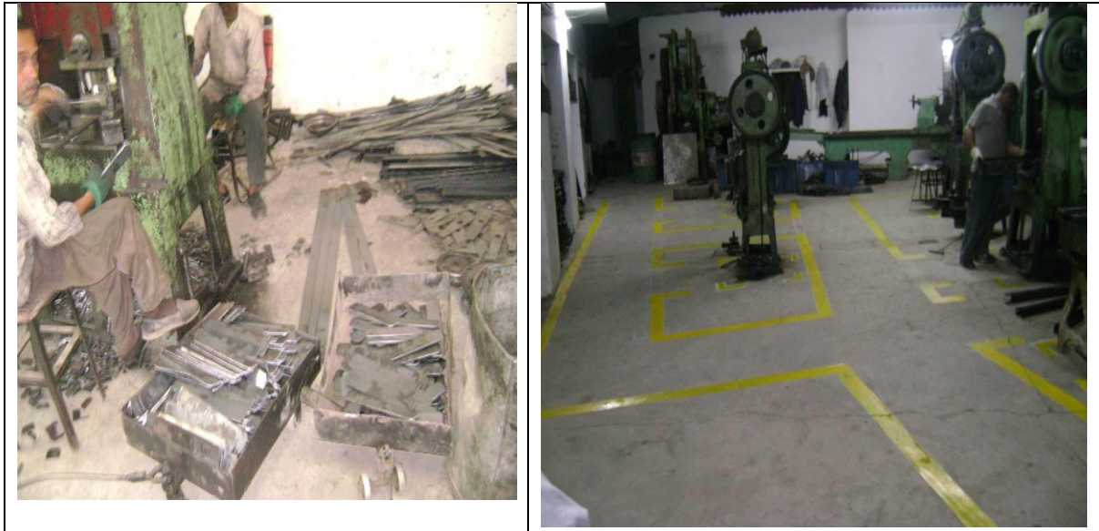
Figure 1: The shop floor was cleaned and a gangway was established through the implementation of KAIZEN principles.
