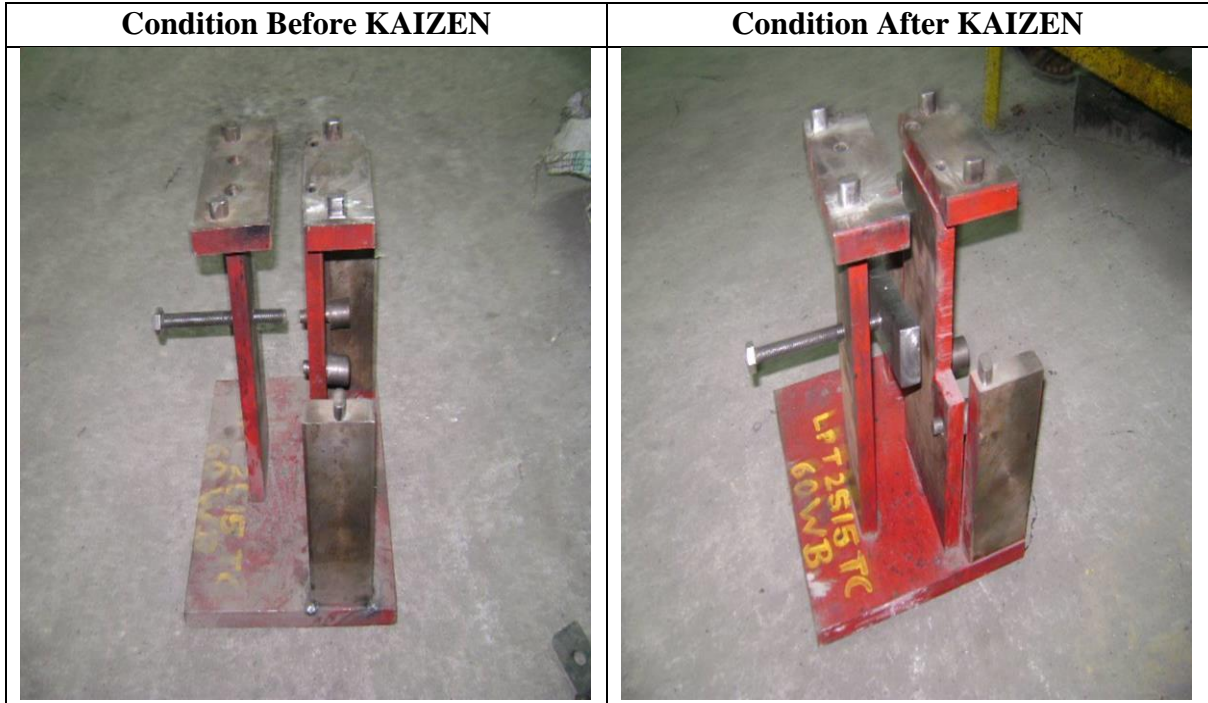
Figure 6: Support plate has been enhanced using the KAIZEN method.
