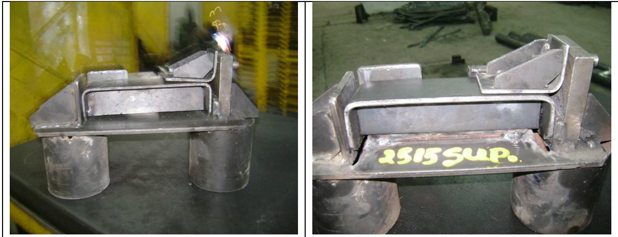
Figure 7: The slot has been improved and the strip welded through the application of KAIZEN principles.
