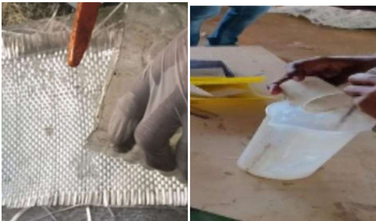
Figure 3. (a) Composite fabrication using Hand lay-up process (b) Mixing of Resin-Hardener-PU
