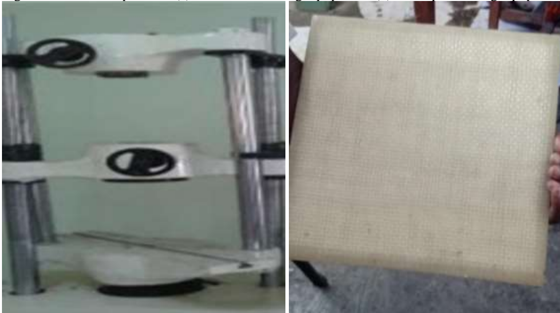
Figure 4. (a) Compression Molding Machine (left) (b) Developed composite (right).
