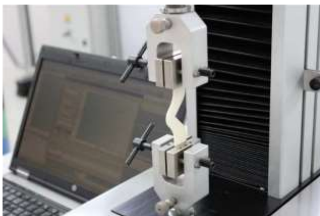
Figure. 2. H-method metal- polymer bitumen device that determines the composition of adhesion.
