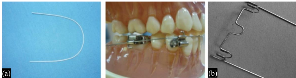
Figure 5. (a) Arc wire and (b) palatal expanders of Nitinol [11, 19].
