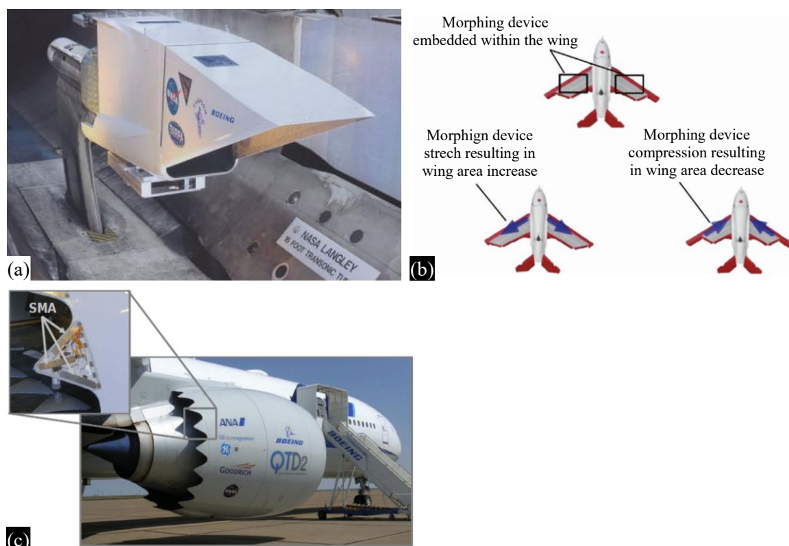
Figure 11. (a) The SAMPSON F-15 inlet tested in the facility at Langley (NASA) (b) Various morphing devices employed on the wing airplanes can change, stretching or compressing, the aerodynamic profile (c) Variable geometry chevron activated by SMA in the full-scale test [26, 27]
