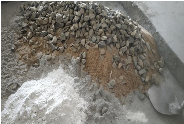
Figure 2. Batching of cement, alccofine, fine aggregate, and coarse aggregate for M60 concrete mix.
