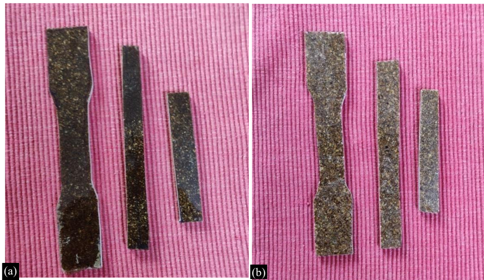
Figure 3. Samples of the desired dimensions for tensile, flexural, and impact tests a) treated composite b) untreated composite.
