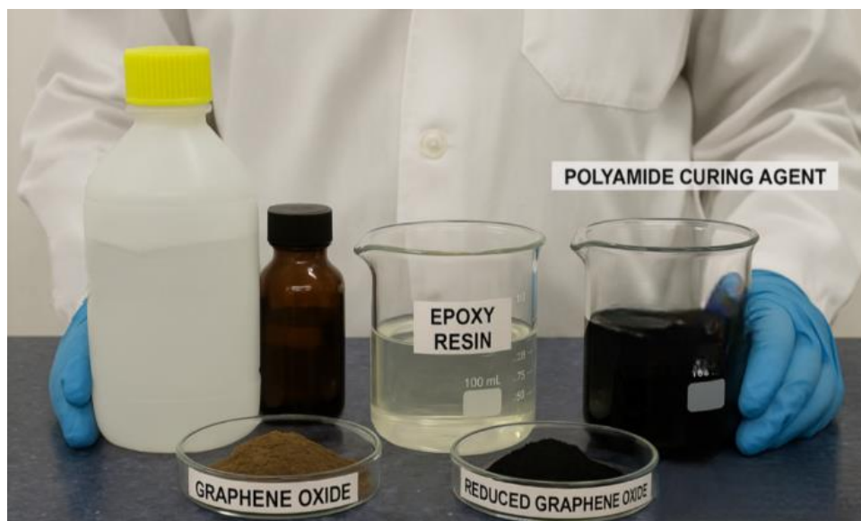
Figure 1. Materials used: epoxy resin, polyamide curing agent, graphene oxide, and reduced graphene oxide.
