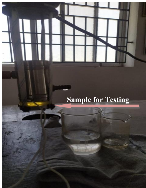
Figure 2. Set up for thermal conductivity measurement. Figure 3. Coir fiber after cutting in desired length
