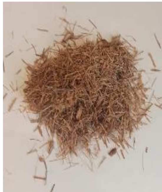
Figure 2. Set up for thermal conductivity measurement. Figure 3. Coir fiber after cutting in desired length
