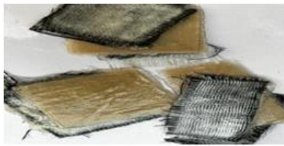
Figure 2. Composite materials before trimming.
