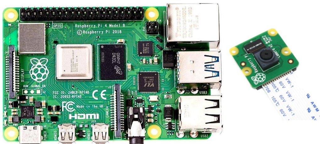
Figure 2. Raspberry Pi 4B and camera module.
