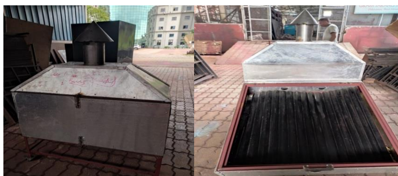
Figure 2. Front and back view of solar dryer.
