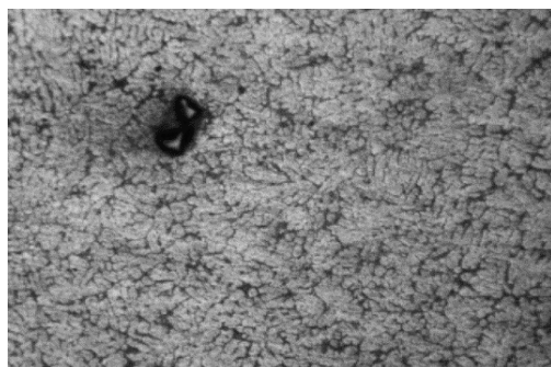
Figure 3. Microstructure of AlSi7Mg0.3/12B 4 C/4ZrO 2 composite (100X)
