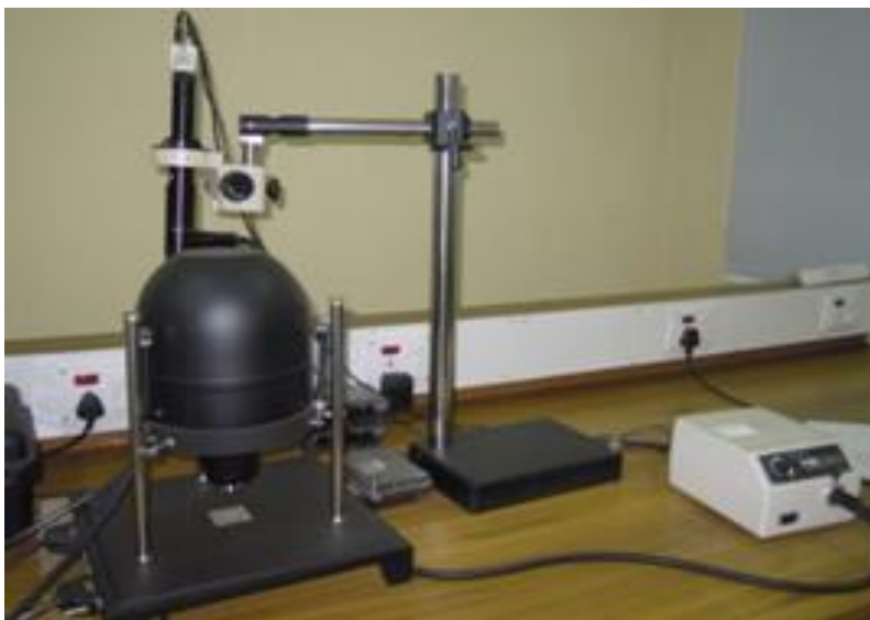
Figure 2. AFM (Model: NT-MDT) Solver-4 used in surface roughness measurement.
