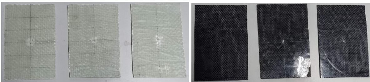
Figure 7. GFRP and CFRP Composite laminates subjected to impact damage.
