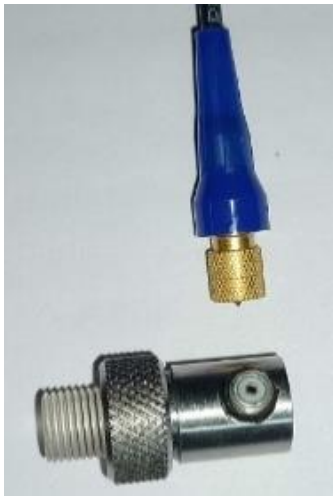
Figure 6. Single crystal wedge delay contact probe of 10.00 MHz frequency.
