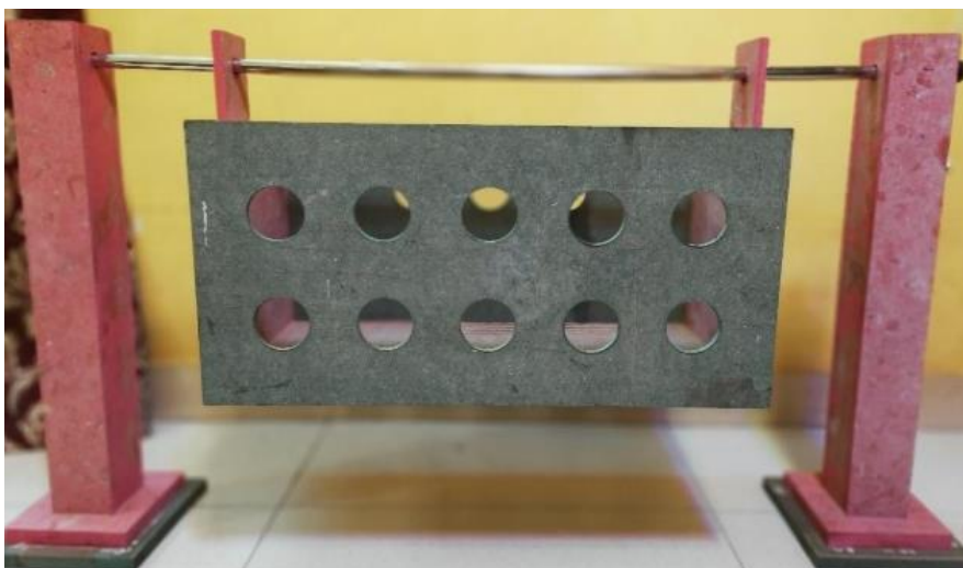
Figure 12. Physical structure of the cradle made from medium-density fiberboard (MDF) wood as wood is not a conducting material.
