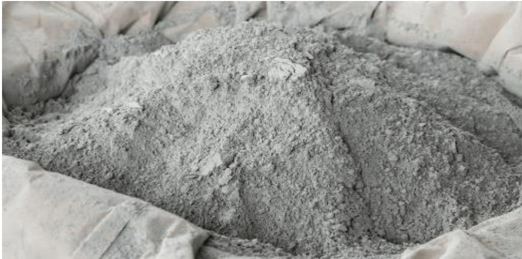
Figure 1. Fly Ash Powder
