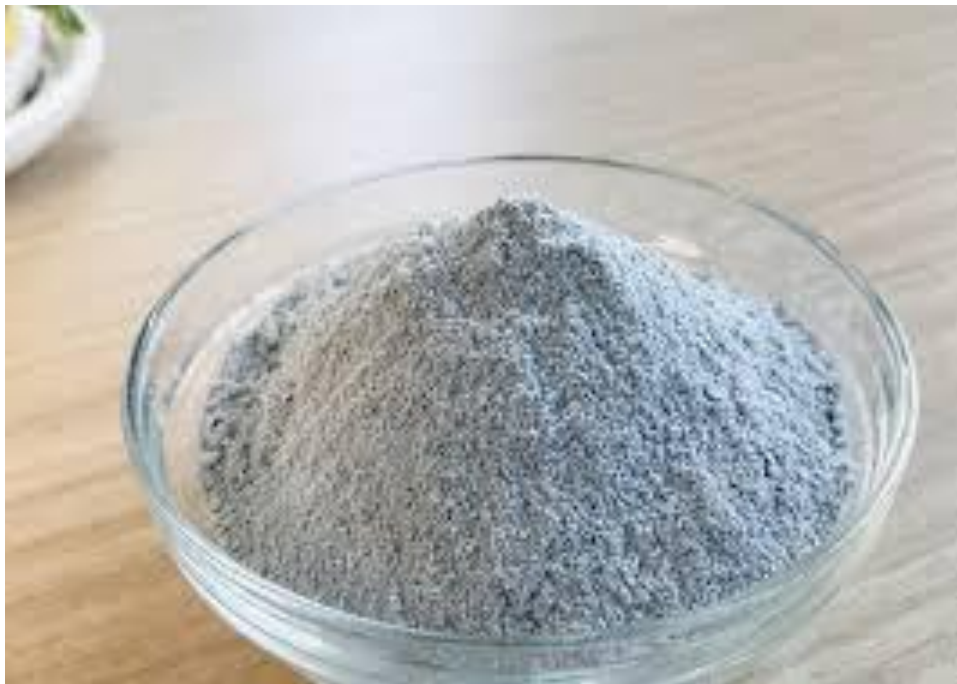
Figure 3. Silica Fume Powder
