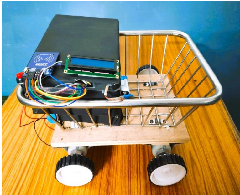
Figure 5. Prototype of smart trolley billing system (implementation).
