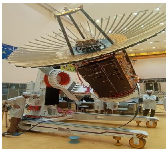
Figure 6. RISAT-2BR1 with its "Radial Rib Antenna" in deployed configuration [3].
