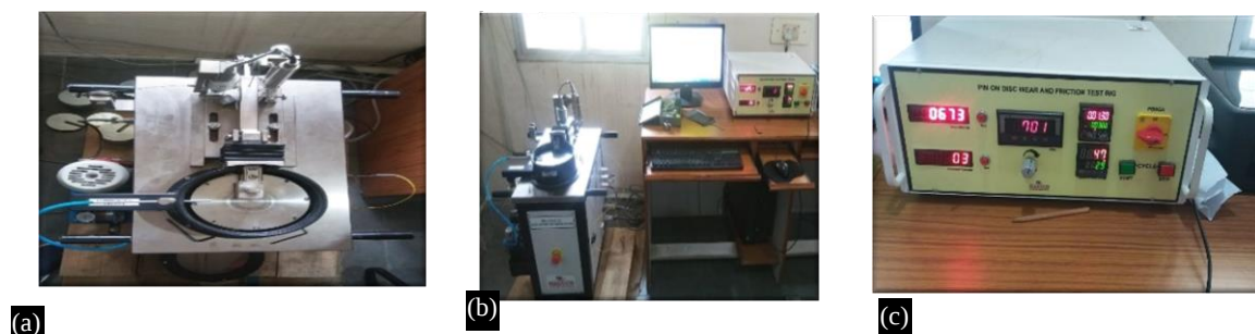
Figure 5. Pin-On-Disc Machine: (A). Top View (B). Landscape View (C). Wear Test Rig.
