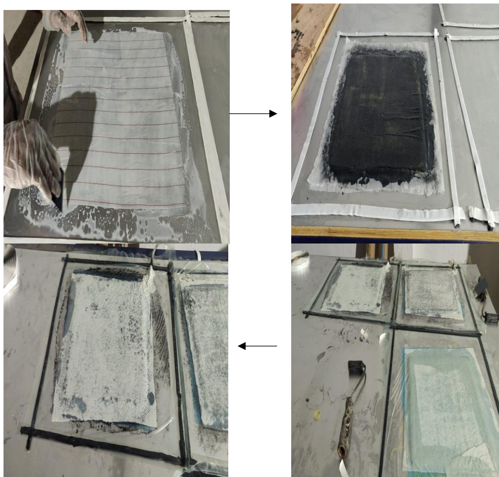
Figure 2. Fabrication sequence of basalt/SS/SiC hybrid laminated composite plates using the vacuum infusion process.
