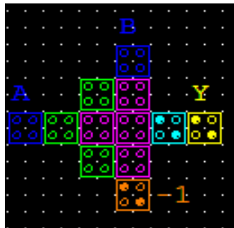
Figure 4. Implementation of 2-input Ex-OR Gate
