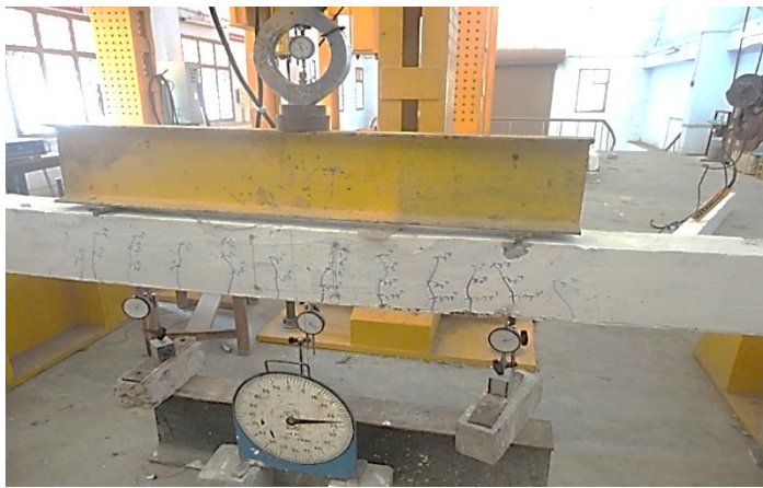
Figure 5. Testing of the beam after cracking.
