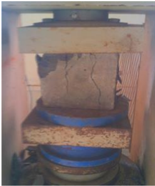
Figure 1. Compressive strength test set-up.
