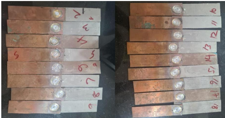
Figure 2. Work pieces before conducting tensile/shear load test.
