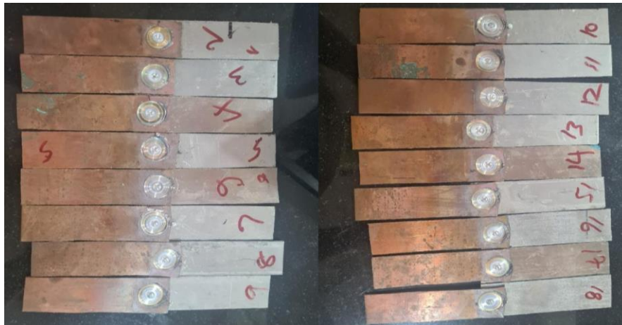
Figure 2. Work pieces before conducting tensile/shear load test.
