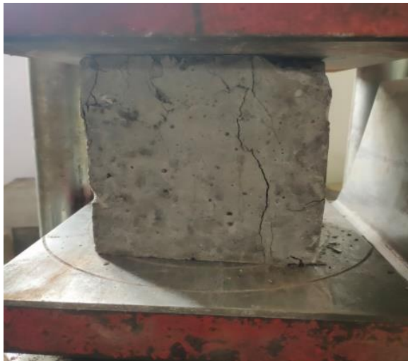
Figure 2. Cracking of GFRc specimen in axial compression.
