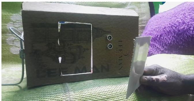
Figure 2. Door closure triggered by absence of nearby object.
