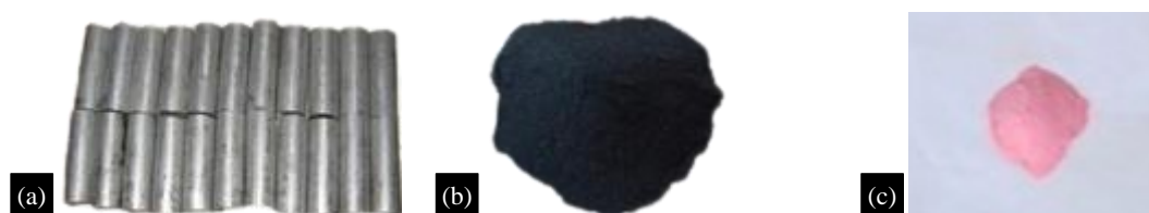
Figure 2. (a) Titanium Matrix Composites (TMCs) Reinforced with Silicon Carbide (SiC), (b) Titanium Matrix Composites (TMCs) Reinforced with Alumina ( \text{Al}_2\text{O}_3 ), (c) Titanium Matrix Composites (TMCs) with Boron Nitride (BN).
