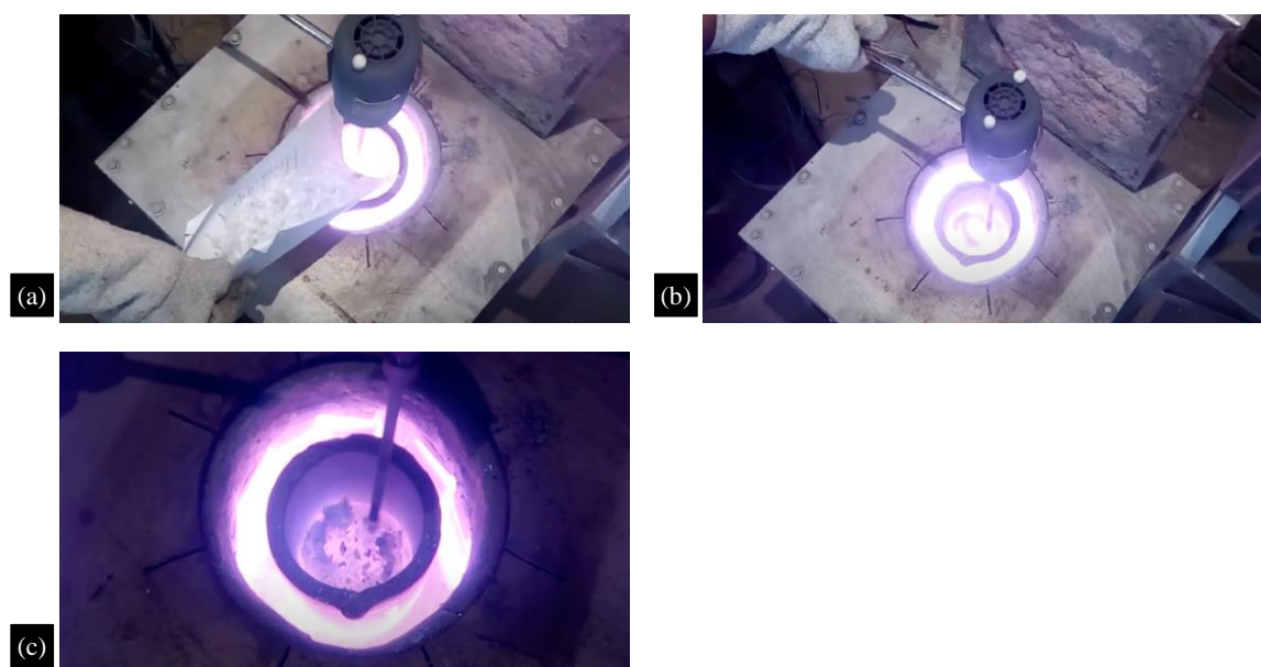
Figure 1. Experimental setup of stir casting Process.
