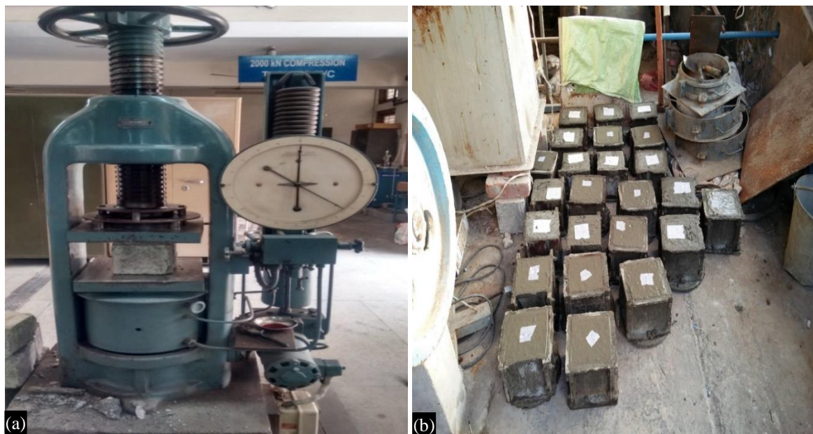
Figure 3. Compressive testing machine and casted cubes. (a) Compressive testing machine; (b) Casted cubes.
