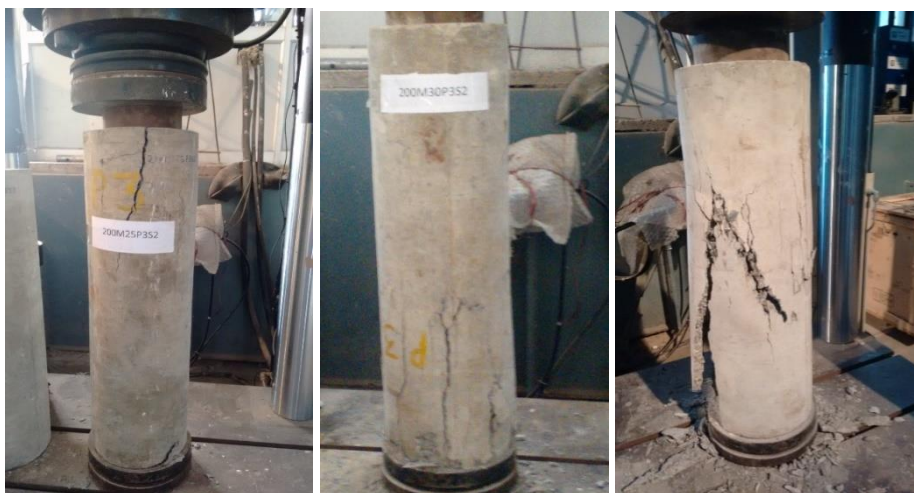
Figure 7. Failure pattern of samples.
