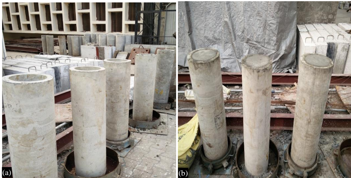
Figure 2. Specimen before and after preparing concrete core. (a) Specimen before preparing concrete core; (b) Specimen after preparing concrete core.
