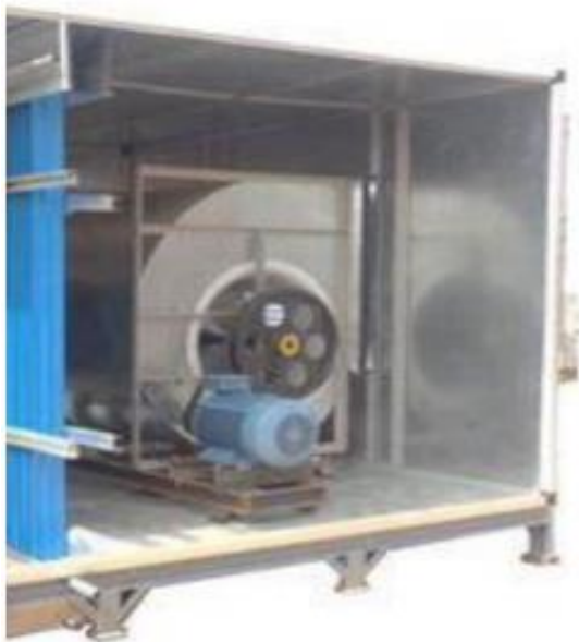
Figure 2. Belt driven blower fan type.
