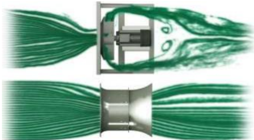
Figure 5. Axial fans utilization of static pressure and dynamic pressure.
