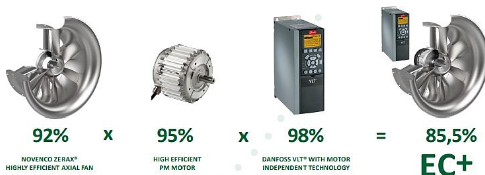
Figure 7. Total Efficiency of EC + fans
