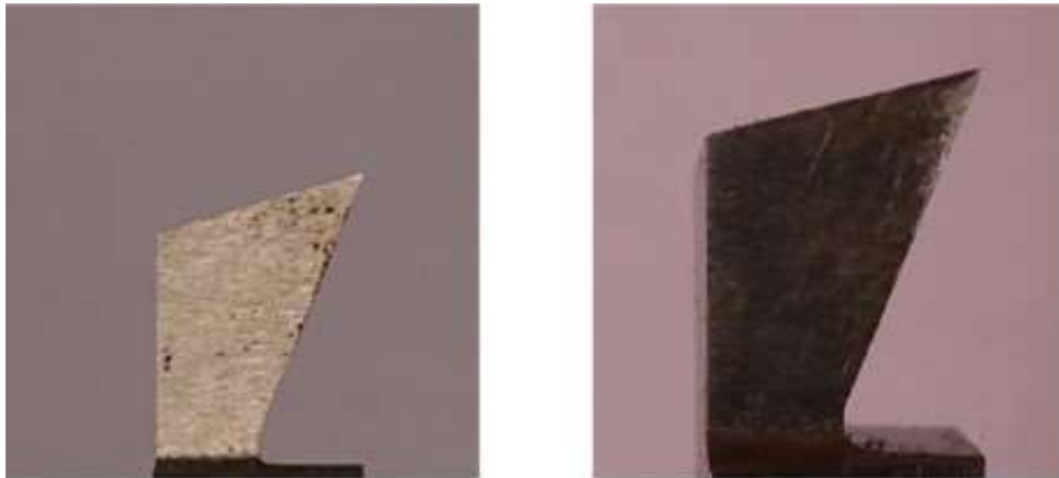
Figure 7. Tool-2(20°) geometry before and after experiment.
