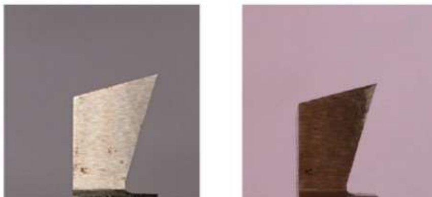
Figure 15. Tool-6(15°) geometry before and after experiment.
