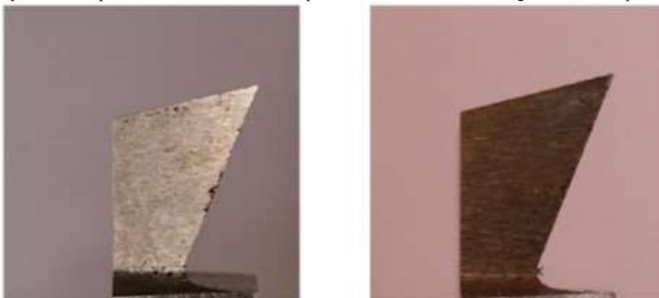
Figure 6. Tool-1(20°) geometry before and after experiment.
