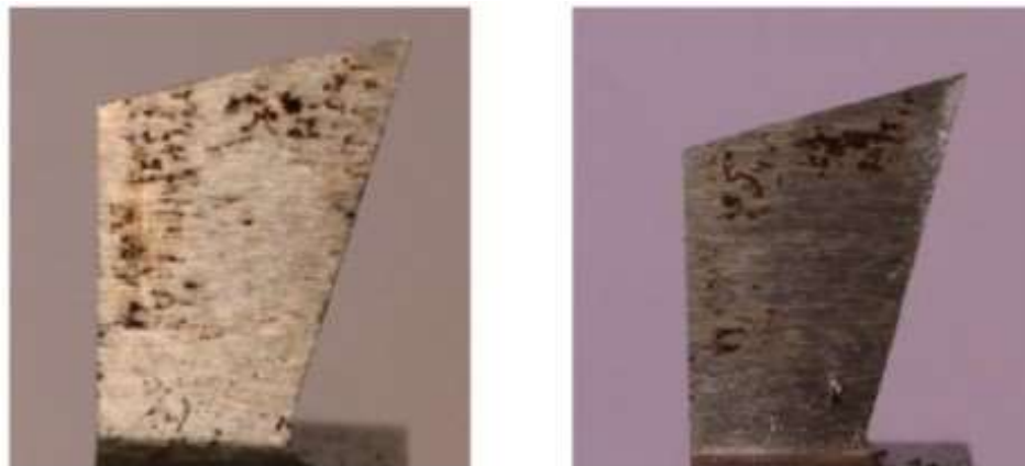
Figure 11. Tool-4(15°) geometry before and after experiment.
