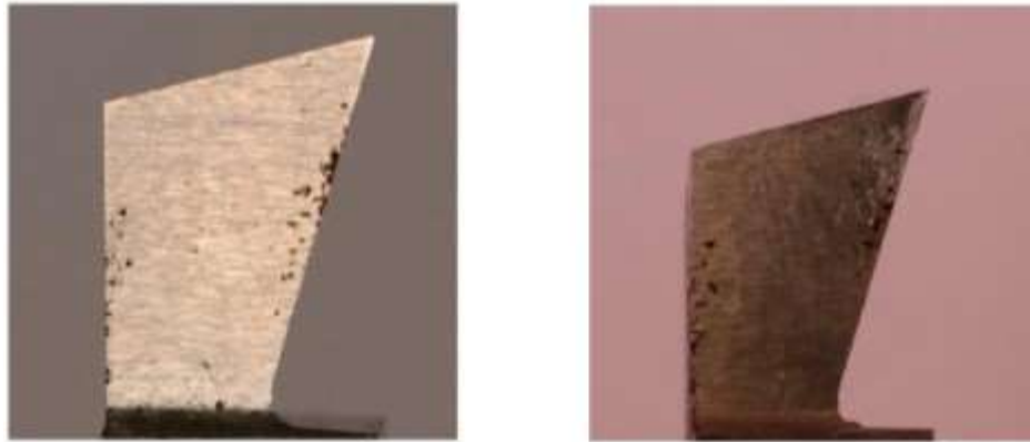
Figure 20. Tool-8(15°) geometry before and after experiment.
