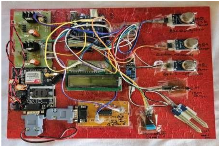
Figure 3. Model of internet of things (IoT)-based environmental monitoring system.
