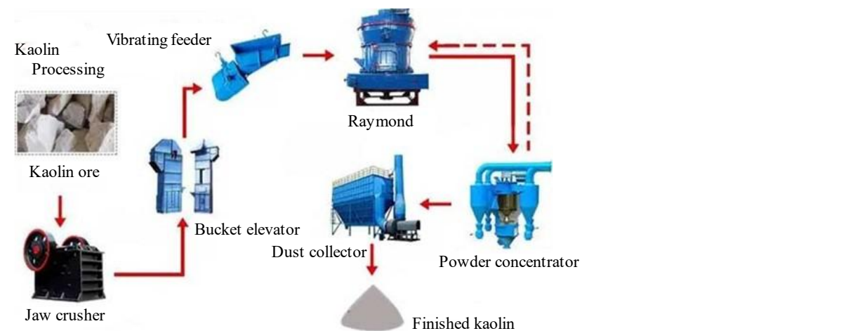
Figure 5. Typical process flow of kaolin manufacturing plant [16].
