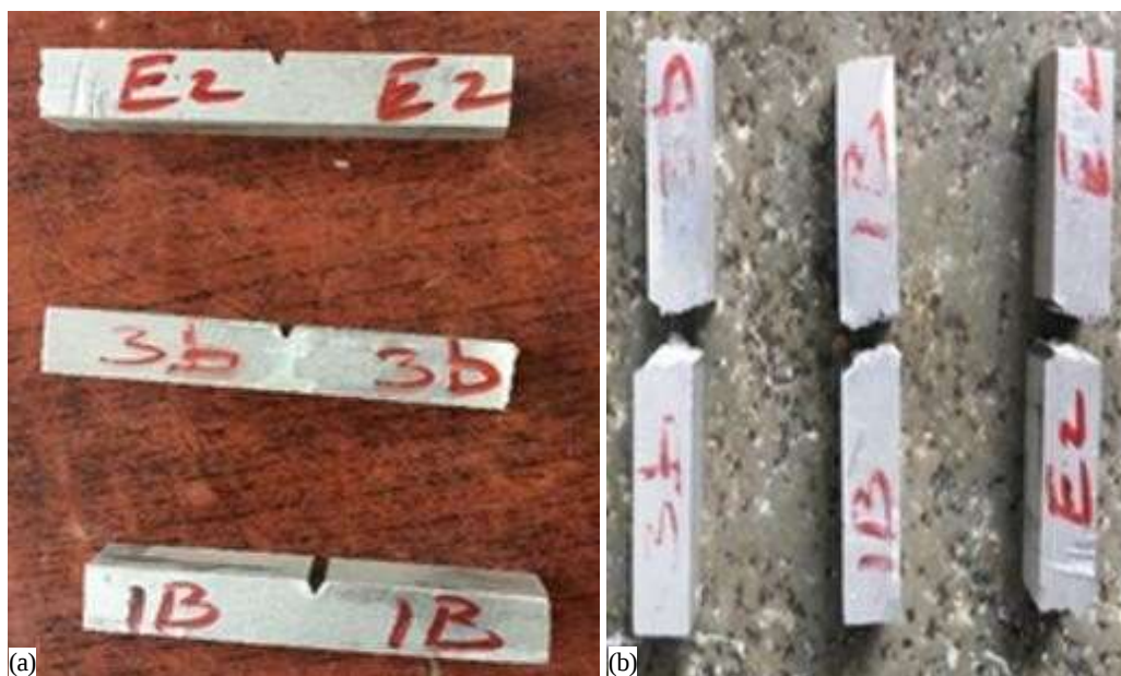
Figure 2. Charpy impact test specimens (a) before testing, (b) after Testing
