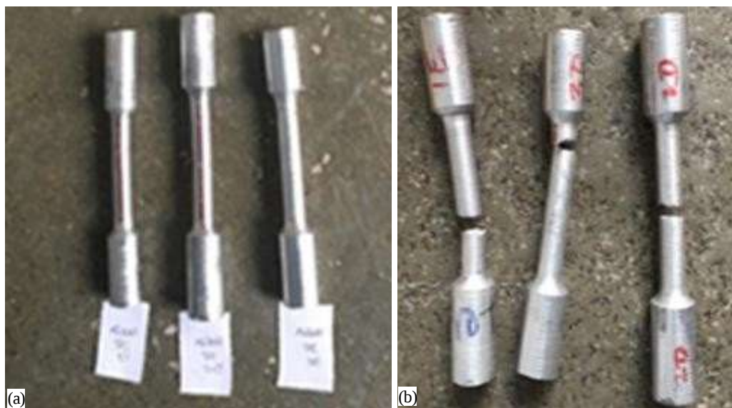
Figure 1. Tensile test specimens (a) before testing, (b) after Testing
