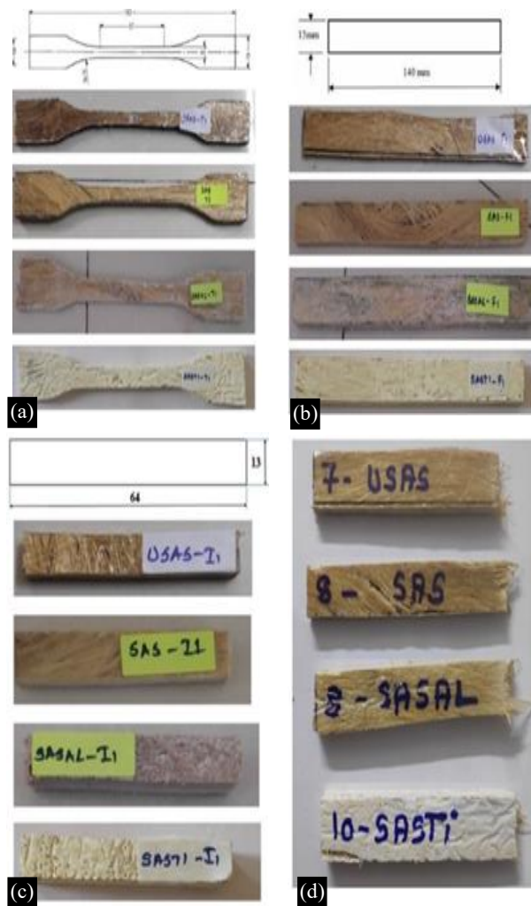
Figure 4. a. Tensile specimen, b. flexural specimen, c. impact specimen. d. shore hardness specimen.
