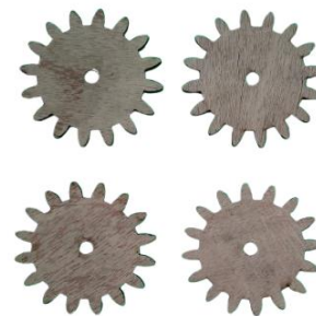
Fig. 2. Four 90mm diameter Planet gear
