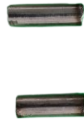
Fig. 4. 200 mm steel rods (8 mm diameter)
