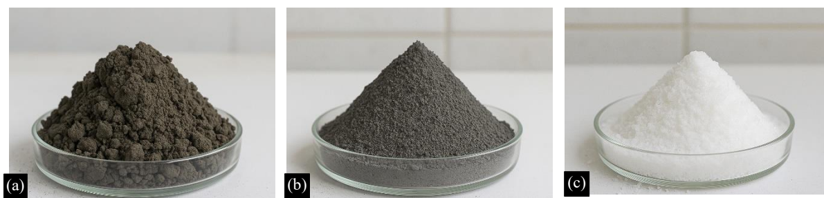
Figure 1. Materials used in the experiments, (a). Black cotton soil, (b). Bagasse ash sample, (c). sodium benzophenone.
