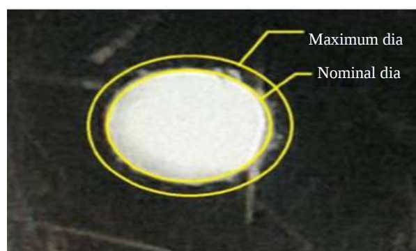
Figure 4. Drilled image of hole.
