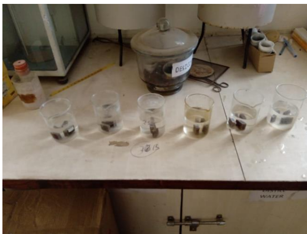
Figure 6. Soaking up of Specimen in Tap Water for Water Take up Test.
