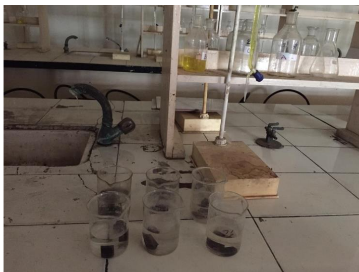
Figure 9. Soaking up of Specimen in Tap Water for Linear Swelling Test [RCERT, Jaipur].
