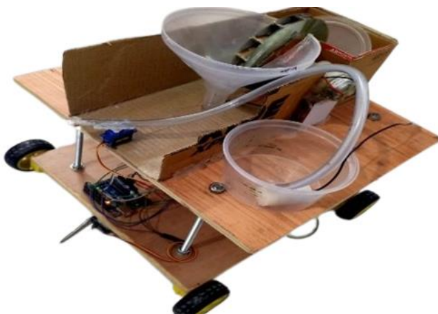
Figure 5. Hydraulic seed covering mechanism.
