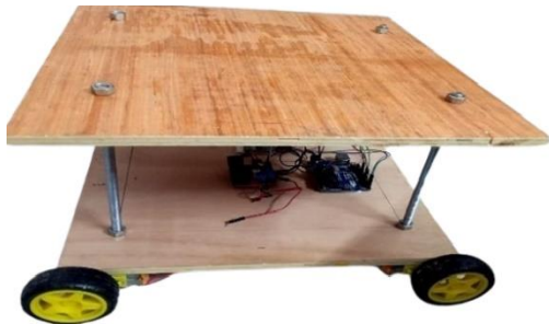
Figure 2. Two-stage adjustable wooden platform with upgraded 12v battery for seed-falling mechanism.
