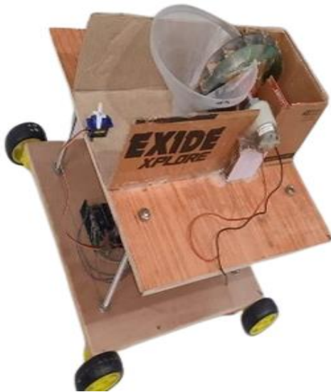
Figure 4. Seed rotation and water sprinkling mechanism.
