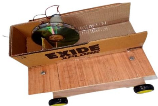
Figure 3. DC motor-driven seed sowing mechanism using rotating disc.
