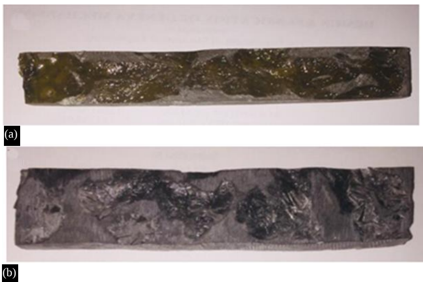
Figure 1. Specimens for tensile testing for a) Glass fiber b) Carbon fiber composites.
