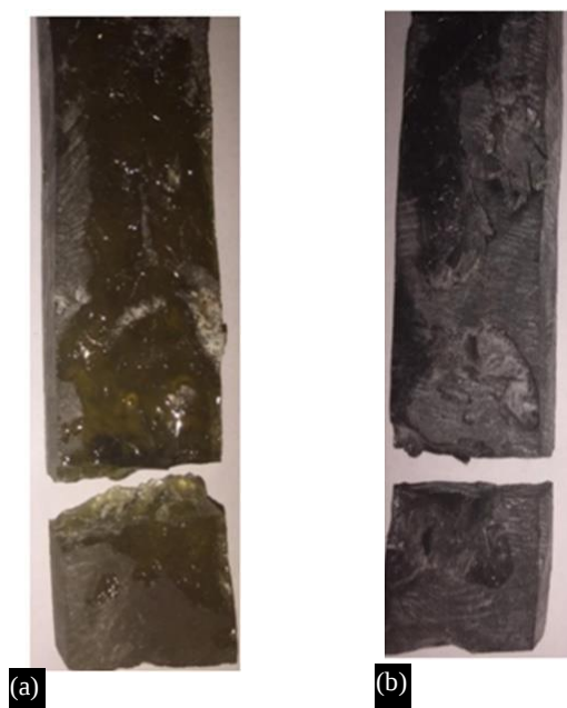
Figure 2. Fractured specimens after tensile testing for a) glass fiber b) carbon fiber composites.
