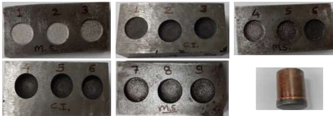
Figure 20. Machined specimens of the MS and cast iron and copper tool.
