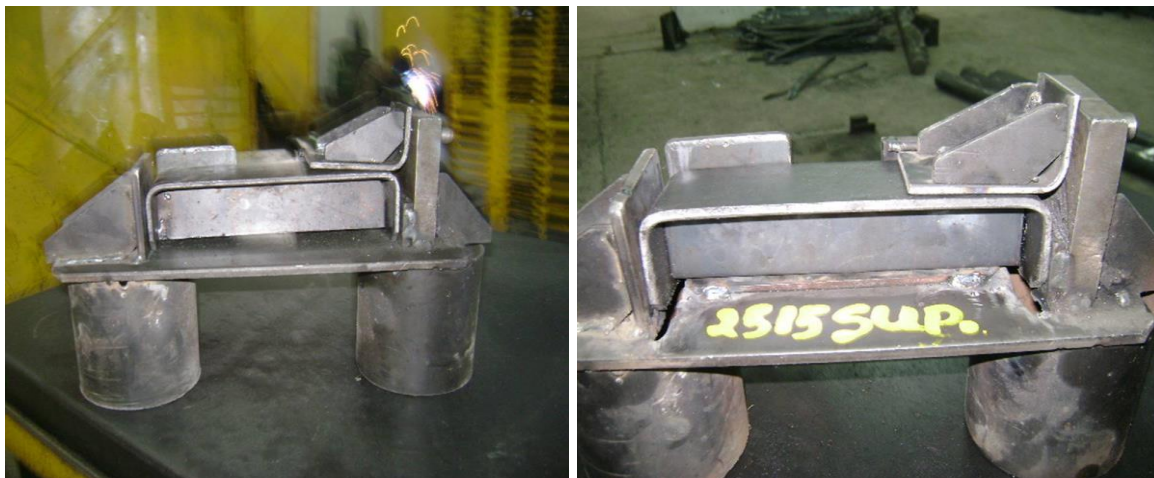
Figure 7. The slot has been improved and the strip welded through the application of KAIZEN principles.
