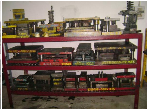
Figure 2. Easy traceability and identification have been improved using the KAIZEN method.
