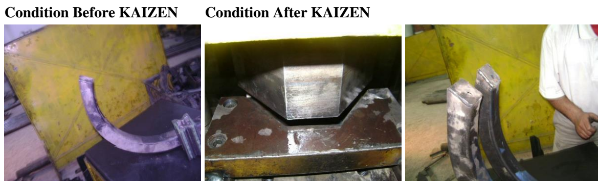
Figure 5. The die angle has been optimized through the application of KAIZEN principles.
