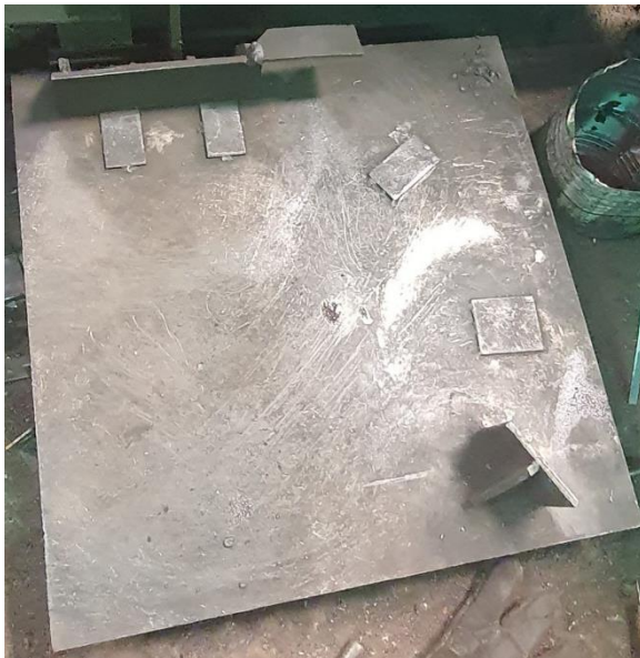
Figure 9. Support plates have been added to prevent workpiece misalignment and distortion.
