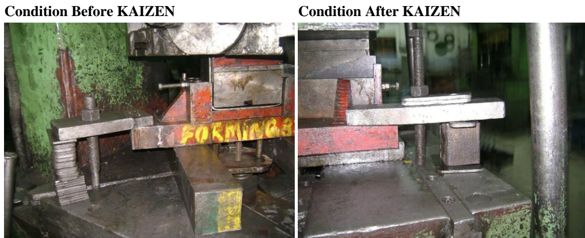
Figure 4. The introduction of clamping blocks instead of packing plates was implemented through the KAIZEN method.
