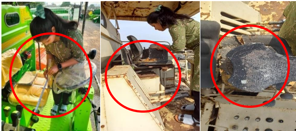
Figure 3. Three-dimensional measurements of controls from seat reference point (SRP).
