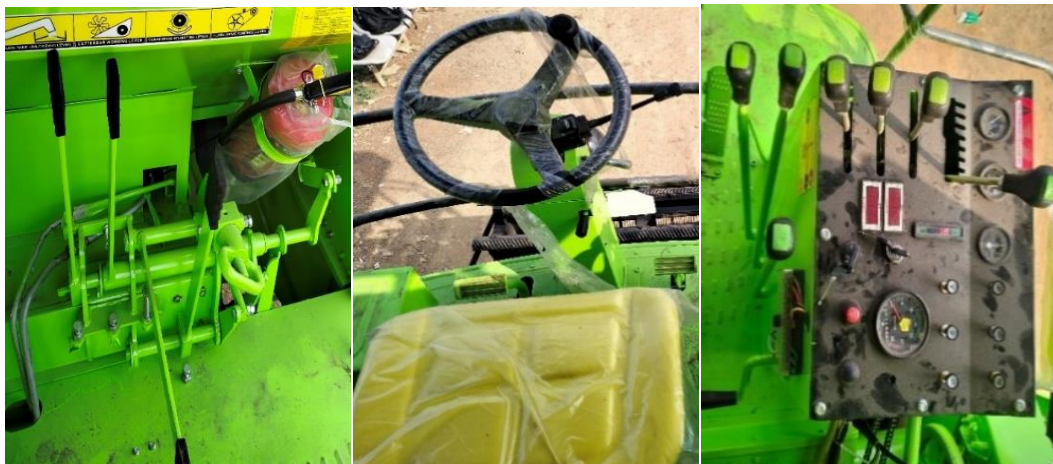
Figure 2. Workplace of combine harvester (left to right): left side, central controls, and right side.
