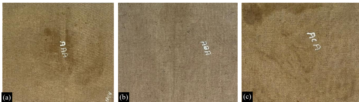
Figure 1. Hybrid composite laminate (a) AAA (b) ABA (c) ACA.
