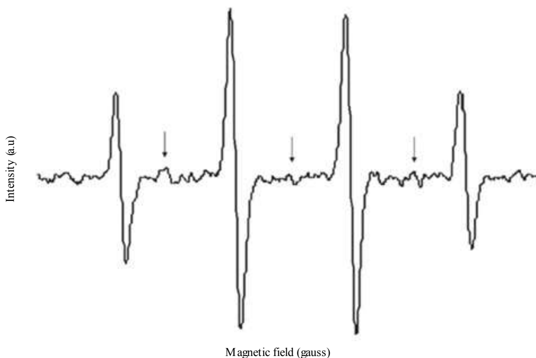
Figure 7. Singlet oxygen production in suspensions of Zn–CuO in the presence of 2, 2, 6, 6-tetra methyl piperidine (TEMP) and 5, 5-dimethyl pyrroline N oxide, DMPO (the triplet of, 2, 2, 6, 6-tetra methyl-1-piperidinyl-oxyl, TEMPO signal formed by the reaction of TEMP with singlet oxygen is marked with arrows). [Reproduced from ref 2 with permission from John Wiley and Sons].
